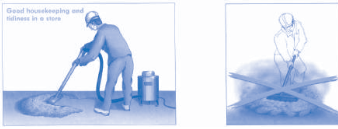
Figure 3.2. Removal of dust deposits (9)
