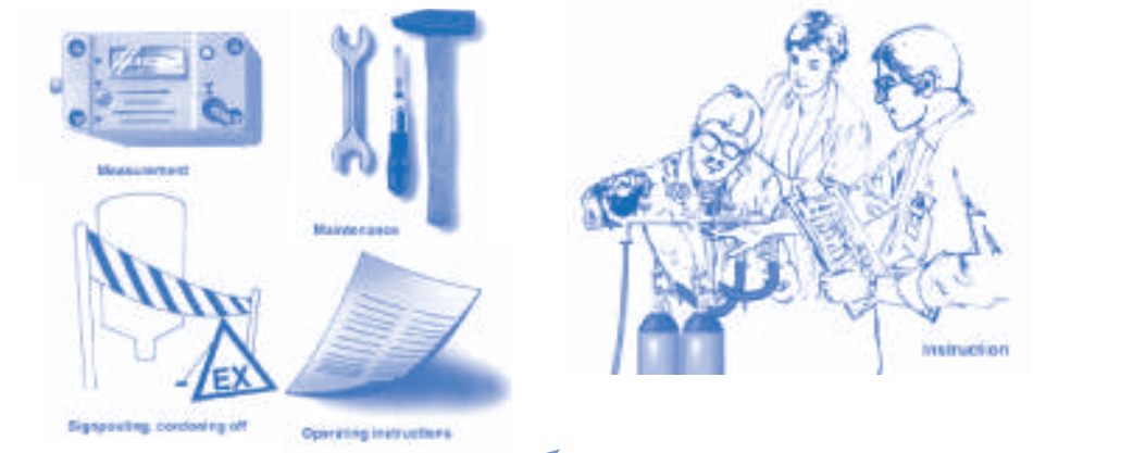
Figure 4.1. Examples of organisational explosion protection measures (12)
