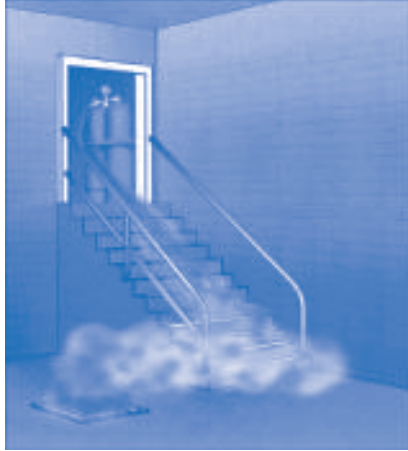
Figure 2.3. Spread of liquefied gases (example) (6)
