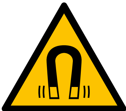
Warning: magnetic field
