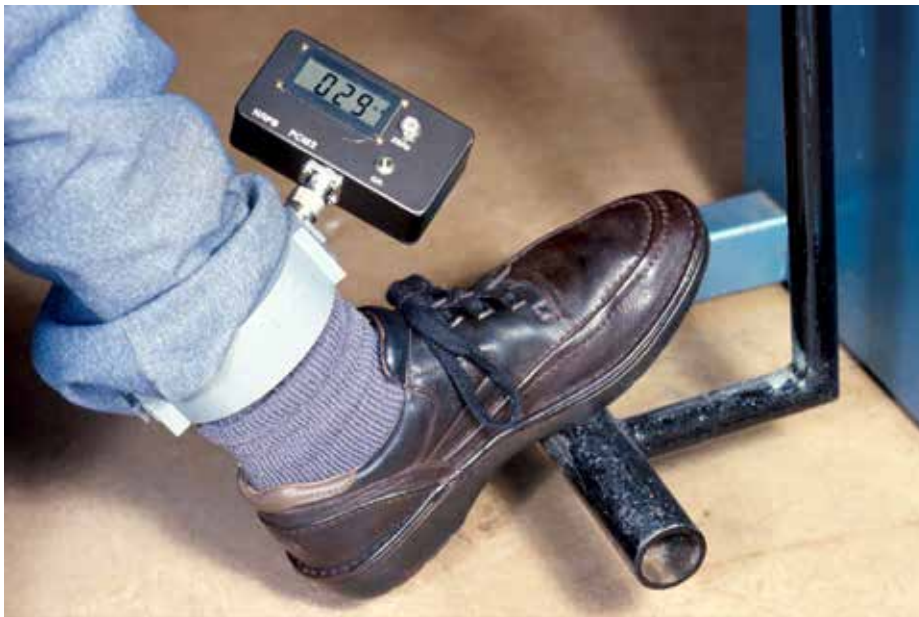
Figure C7 — A current clamp being used to measure the limb current when using a 27 MHz dielectric welder
