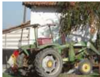
Tractor with rollover protection bars
